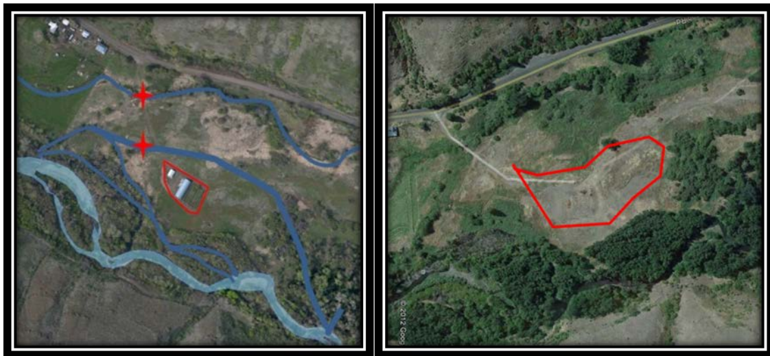
Figure 9. Project Area 18 floodplain restoration project. Image A illustrates the pre project condition. The blue lines on the image indicate the over land flows which occurred in 2009 and 2010. The red polygon highlights the infrastructure removed as part of this project. Image B illustrates the post project condition of the site in September 2012. The red polygon indicates the position of the removed infrastructure.
